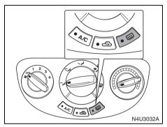
The rear window defogger uses a warming grid to remove fog or frost from the rear window. This feature will only work when the ignition is in ON.
